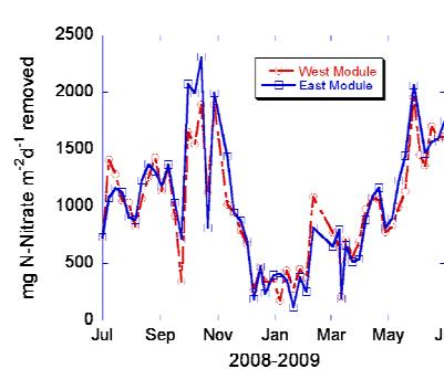
**Figure 2:** nitrate removal efficiency by CAS fed with secondary-treated MWE
