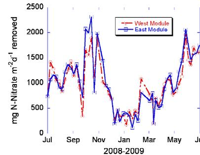
Figure 2: nitrate removal efficiency by CAS fed with secondary-treated MWE
