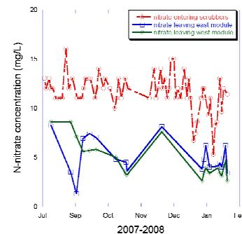
**Figure 1:** nitrate removal by CAS fed with tertiary-treated MWE
